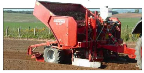
Robust example: The 2-row GL 32 T was developped on the basis of the successful model GL 34 T. Thanks to the very stable and compact frame, the bunker can hold up to 2,500 kg.
