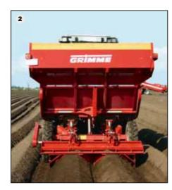
Grimme has always put emphasis on economics. Therefore we offer bunker models that are selectable according to your requirements. The standard bunkers has a capacity of 1,000 kg and can be extended to 1,200 kg (1) with a rubber ledge. For all who wish to increase their output with a larger bunker capacity and who wish to save time by less filling procedures, the 2.45 m wide large bunker with a capacity of 2,200 kg (2) is the first choice.
