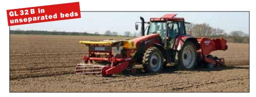
Fertilizing, planting, ridge forming: With the GL 32 B, you can achieve everything in one work step – even on unseparated surfaces. The cooperation of the compact GL 32 B and the optional fertilizer unit in the front allows for extremely quick turning manoeuvers. This way, you do not lose time and profit from quick results.
