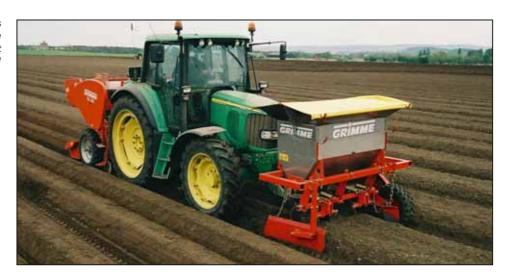
Solid preparation work: The front cultivator forms the ridges in front of the tractor, so that as little soil as possible becomes compacted.
