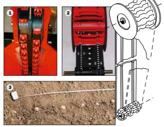
Small details which make a big difference: The large diameter upper pulley (1) ensures a positive drive and safe delivery, even with long potatoes. It also gives correct belt guiding. Two reinforced guiding ribs (2) behind the belts ensure a reliable alignment, even with oversized potatoes at the upper pulley. And the smaller belt pulley (4) at the bottom guarantees a fast opening and therefore a good delivery (3).
