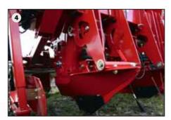
This will leave even light soils in great shape for a long time: The large sized tines of the covering bodies assembly (3) are used to form the ridge. The bulbous shape is created by a light solidification of the soil with the cage roller, which still allows the surface to remain rough.
