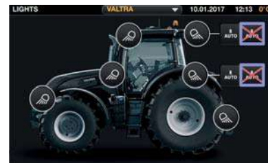
Easy configuration of worklights from the terminal. Worklights on/off switch in the armrest with beacon on/off switch.
