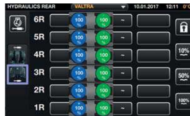
From any control you can control any hydraulic service including hydraulic valves (front and rear), linkages (front and rear) or front loader
