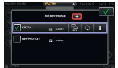
Profiles for operators and implements which can be easily changed from any screen menu. All the setting changes will be saved in the selected profile
